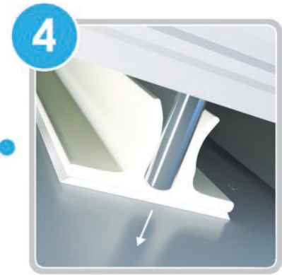
4 Lock die into press and index machine to place Matrix on opposing platen
